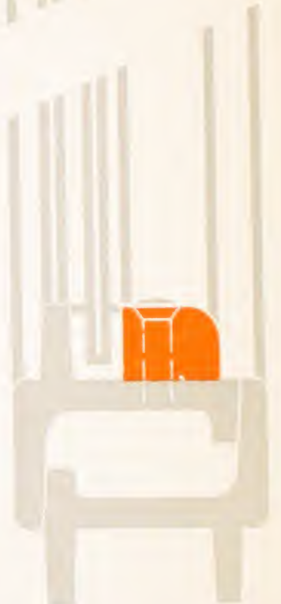
STEEL BEAD APPLIED TO SMALL SECTION
